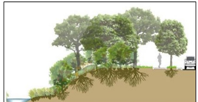
Roots from shoreline vegetation filter pollutants (including sediment and nutrients) and slow the flow of stormwater runoff to the waterbody. Shade provided by the vegetation cools the water temperature and provides benefits for birds and wildlife.
